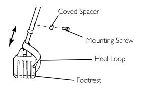
FIGURE 6.5 Footrest Height Adjustment - 70° Taper
